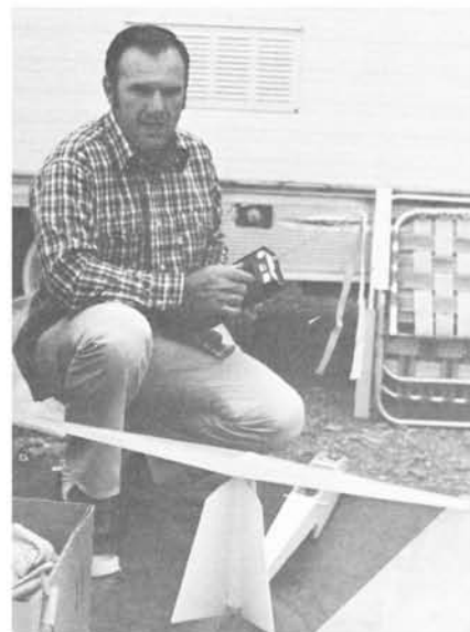
Joe McClaran's original "Split Tee" design that he flew at the 1975 LSF Tournament at Mile Square Park in So. Cal. Features the dive brake/spoiler shown in Fig. 6 below. Joe reports that at less than full separation, there is still directional control. Photo by Taylor Collins.
