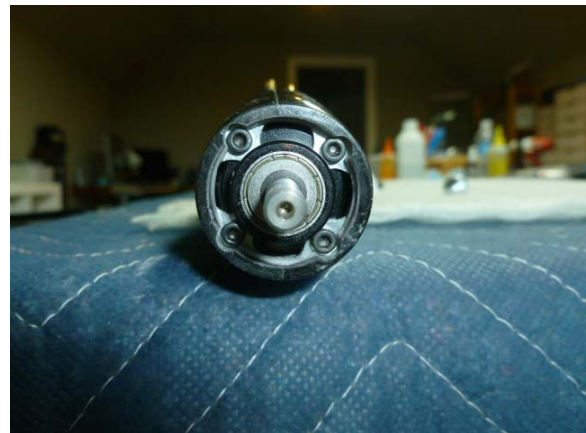
You can see the relief areas needed for the motor screws.
