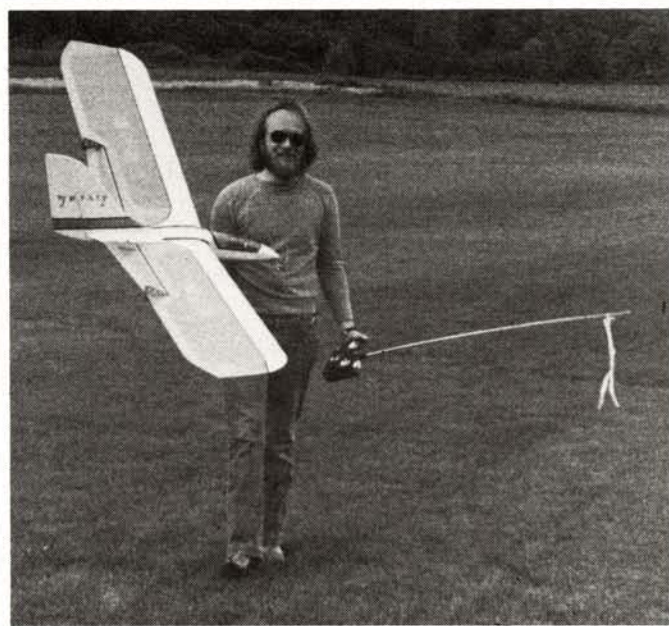
Ken Bates with the Windlord. Sweepback not essential in a flying wing.
